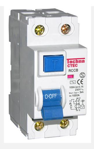
A RCD (Residual Current Device) is a safety device that disconnects a circuit when it detects an imbalance of the electric current. The RCD turns the power off almost immediately to prevent electrocution. While you may still receive an electric shock, the duration will be very short, reducing the risk of serious injury.
