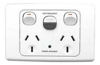
RCDs may be fitted to a power point, and can be distinguished by the test button on the faceplate. They must be fitted to the first power point after the meter box. They are suitable for protecting electrical appliances in specific areas such as bathrooms and workshops.
